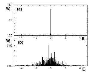
FIG. 3. Two quantum computer eigenstates of model (1) in the basis of noninteracting multiqubit states, i.e.,  $W_i = |\langle \psi_i | \phi \rangle|^2$  as a function of noninteracting multiqubit energy  $E_i$  for n = 12 and  $\delta = \Delta_0$  with  $J_c / \Delta_0 = 0.273$  (see text): (a)  $J / \Delta_0 = 0.02$ ; (b)  $J / \Delta_0 = 0.48$ .
