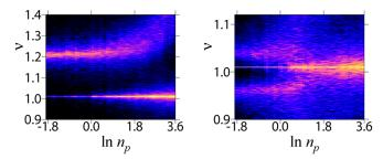
FIG. 6 (color online). Spectral density  $S(\nu)$  of qubit radiation  $\xi_z(t)$  as function of driving power  $n_p$  in the presence of phase noise in  $\phi$  with diffusion rate  $\eta = 0.004\omega_0$ . Left:  $\Omega/\omega_0 = 1.2$ ; right:  $\Omega/\omega_0 = 1$ . Other parameters are as in Fig. 1. Grayness (color) shows  $S(\nu)$  in logarithmic scale [white (black) for maximal (zero)],  $\nu$  is given in units of  $\omega_0$ .
