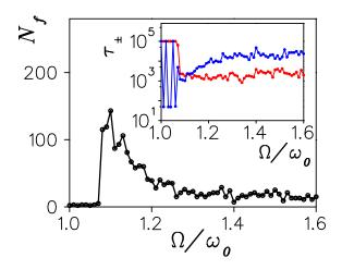
FIG. 5 (color online). Dependence of number of transitions  $N_f$  between metastable states on rescaled qubit frequency  $\Omega/\omega_0$  for parameters of Fig. 1;  $N_f$  are computed along 2 QT of length  $10^5$  driving periods. Inset shows lifetime dependence on  $\Omega/\omega_0$  for two metastable states [ $\tau_+$  for gray (red),  $\tau_-$  for black (blue),  $\tau_{\pm}$  are given in number of driving periods; color choice is as in Figs. 2 and 3].
