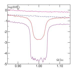
**Figure 3.** Dependence of the rescaled diffusion rate  $D/D_0$  on the rescaled frequency  $\Omega/2\omega$ . The full curves are for  $\epsilon = 0.64$  with  $N_{cel} = 50 \times 50$ ,  $100 \times 100$ ,  $200 \times 200$  from top to bottom; the dashed curve is for  $\epsilon = 0$  and  $N_{cel} = 100 \times 100$ . Data are obtained for time  $t \le 10^4/\Omega_s$ , N = 1000. Logarithms are decimal.
