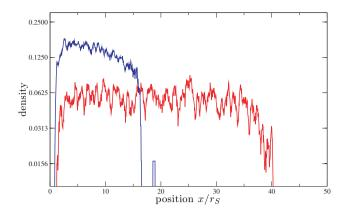
**Figure 7.** Dependence of density of particles (arbitrary units in logarithmic scale) on position in the ring  $x/r_s$  for  $\epsilon = 0.6$  at the final time  $\Omega_s t = 6.28 \times 10^4$  (red/grey for parameters of Fig. 5) and  $\Omega_s t = 6.28 \times 10^5$  (blue/black for parameters of Fig. 6).
