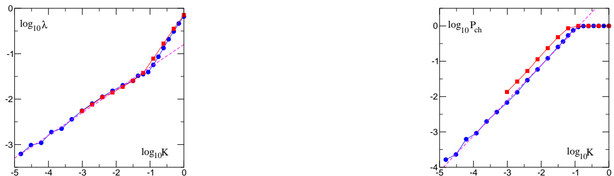
Fig. 5 Left panel: Dependence of the Lyapunov exponent \lambda on the perturbation parameter K for model A at L = 4 (blue circles), 8 (red squares). Dashed straight line shows approximate dependence \lambda = 0.16\sqrt{K} (for N = 4, 8 ). The fit of data gives the exponent of the dependence \lambda \propto K^a with a = 0.476 \pm 0.013 (for L = 4 ), 0.450 \pm 0.012 (for L = 8 ) in agreement with the scaling (5). Right panel: Dependence of the measure of chaos P_{ch} on the perturbation parameter K for L = 4 (blue circles), 8 (red squares). Dashed straight line shows approximate dependence P_{ch} = 7.75K (for L = 4 ); for L = 8 we find that P_{ch} = 14.32K in agreement with the scaling (4). The fit of data gives the exponent of the dependence P_{ch} \propto K^b with b = 1.022 \pm 0.01 (for L = 4 ), 1.036 \pm 0.01 (for L = 8 ). Up to 5 \times 10^5 trajectories and time t \leq 10^6 have been used to compute the Lyapunov exponent \lambda and determine the number of chaotic trajectories with \lambda > 0 . Certain checks have been made with t = 5 \times 10^9 and 100 trajectories.
