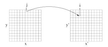
FIG. 8 Illustration of operation of the Ulam method: the phase space (x, y) is divided in  $N = N_x \times N_y$  cells,  $N_c$  trajectories start from cell j and the number of trajectories  $N_{ij}$  arrived to a cell i from a cell j is collected after a map iteration. Then the matrix of Markov transitions is defined as  $S_{ij} = N_{ij}/N_c$ , by construction  $\sum_{i=1}^{N} S_{ij} = 1$ .
