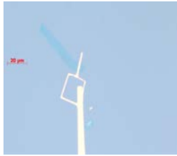
few (?) layer graphene on Si/SiO 2
