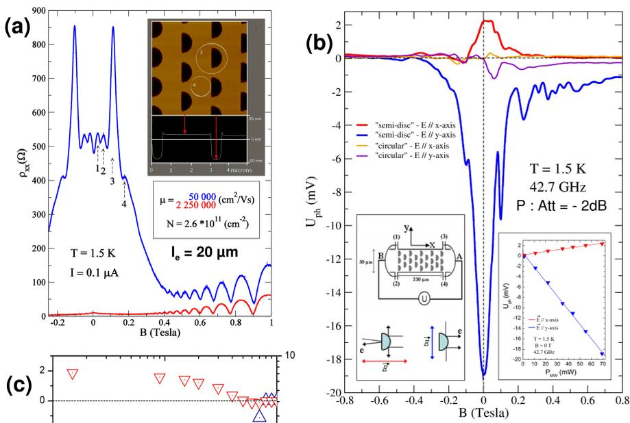
Samples are high mobility 2DEG based on AlGaAs/GaAs heterostructures with Hall bar geometry. The lattices of semicircular antidots fabricated by EBL and plasma etching have the dimensions  $250 \times 50$   $\mu\text{m}^2$  and the parameters: period =  $1.5$   $\mu\text{m}$  and antidot radius =  $0.5$   $\mu\text{m}$ . Lattices with the same parameters but with circular antidots were also fabricated.
