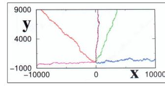
Large scale: linear trajectory. Directed transport for one trajectory at various polarizations of radiation:  $\alpha = 0, \pi/8, 0.21\pi, \pi/4, \pi/2$  (from left to right clockwise).
