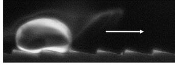
Directed motion of a water droplet created by heating of the asymmetric metallic surface.
