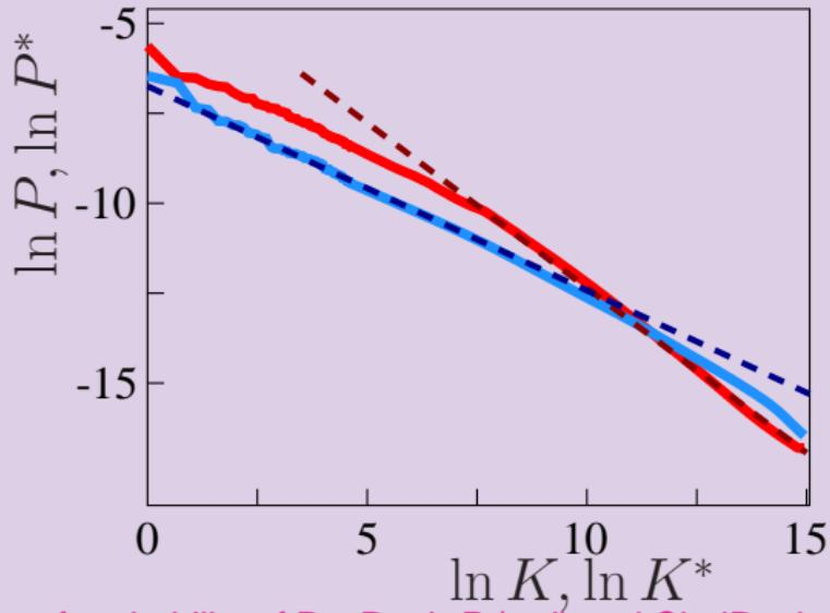
Dependence of probability of PagRank  $P$  (red) and CheiRank  $P^*$  (blue) on corresponding rank indexes  $K, K^*$ ; lines show slopes  $\beta = 1/(\nu - 1)$  with  $\beta = 0.92; 0.57$  respectively for  $\nu = 2.09; 2.76$ .
