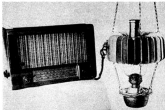
Oil burning lamp powering a radio using
