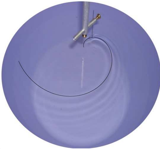
FIG. 3: (Color online) Photography of the wave crests generated on a water surface by a needle rotating counterclockwise along a circular trajectory (radius \mathcal{R} \approx 2.7 \text{ cm} \approx 9 \kappa^{-1} ) with a velocity V \approx 21 \text{ cm} \cdot \text{s}^{-1} \approx 0.9 c_{\min} . The black curve represents the predicted Archimedean spiral with radius a given by Eq. (8).
