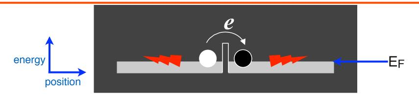
After tunneling event, spreading of charge inhibited by environment
