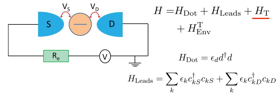
Need quantum description of <u>electrical</u> properties of the junctions S and D, i.e. a **quantum capacitor**:  $e^{-\int_{-\infty}^{t}}$
