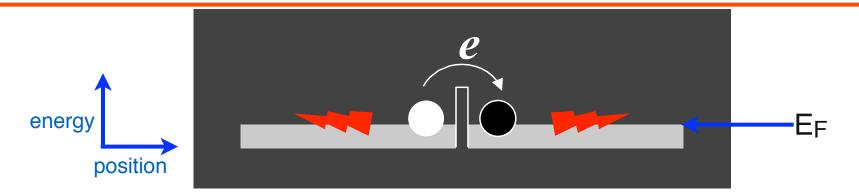
After tunneling event, spreading of charge inhibited by environment
