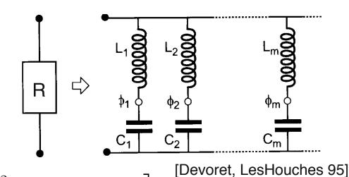
$$H_{\text{Env}}^{\text{T}} = \frac{q^2}{2C} + \sum_{m} \left[ \frac{q_m^2}{2C_m} + \left(\frac{\hbar}{e}\right)^2 \frac{1}{2L_m} \left(\varphi - \varphi_m\right)^2 \right]$$
