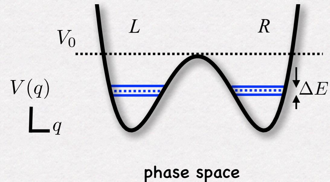
A period of the tunneling oscillation between symmetric wells
